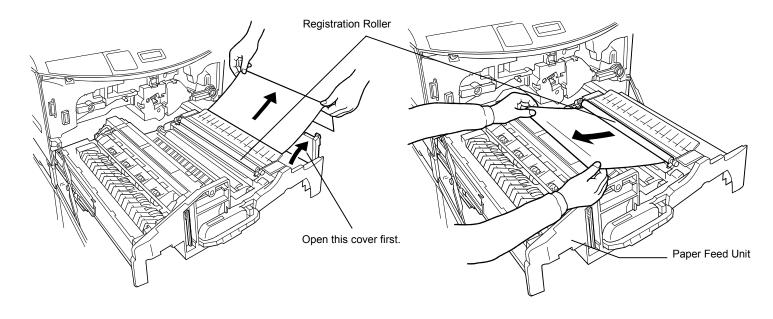
Figure 5.3. Paper jammed in paper feed unit
